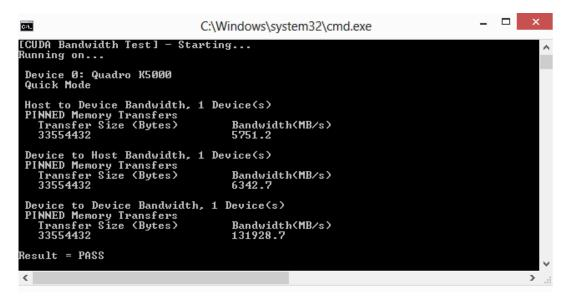
Figure 2: Valid Results from bandwidthTest CUDA Sample
