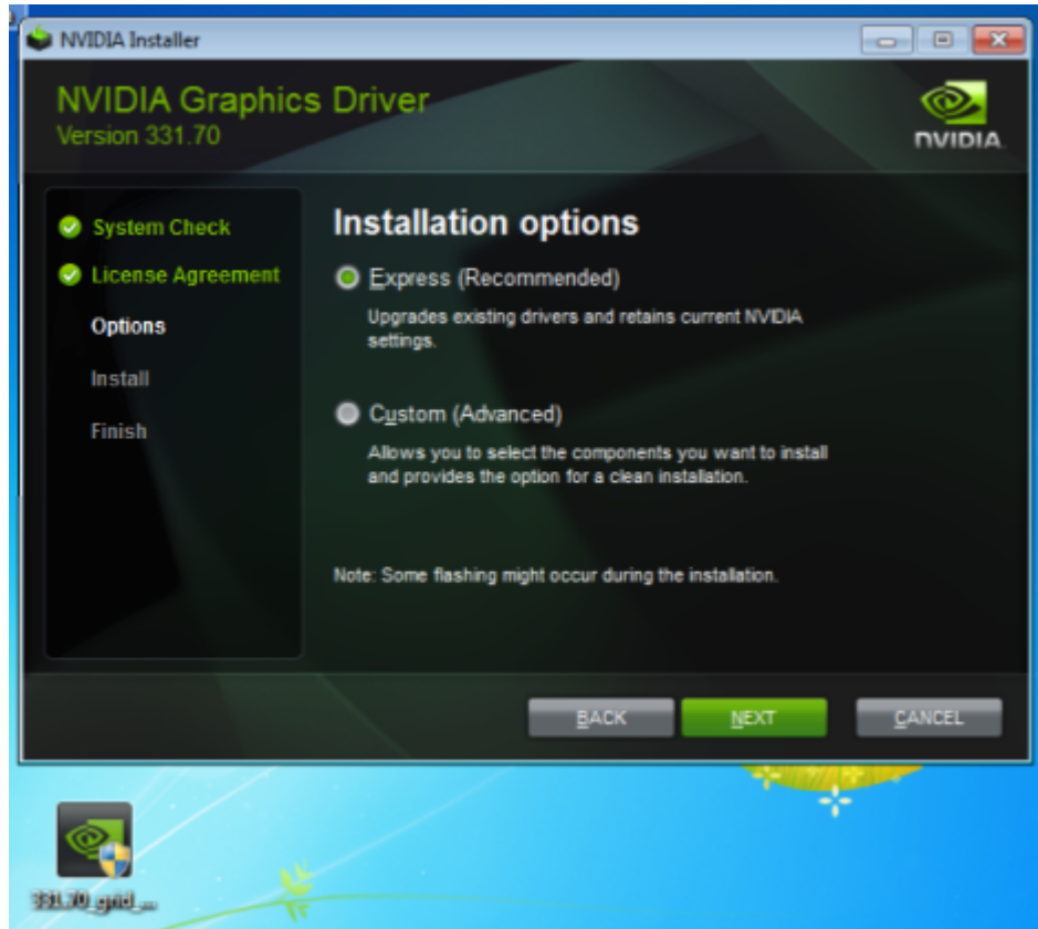
Figure 14 NVIDIA driver installation in the guest VM
