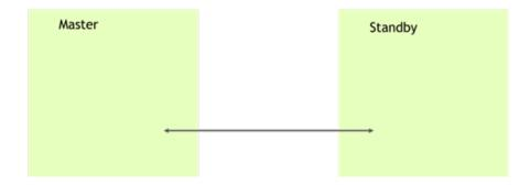
UFM-HA employs a dual-link configuration comprising primary and secondary connections to enhance system stability while mitigating the risk of connectivity challenges. It leverages two prioritized IP addresses, primary and secondary, which the Pacemaker utilizes to establish two connectivity links. Notably, DRBD utilizes the primary IP address to synchronize data. It is recommended to utilize this IP address for interfaces with high transfer rates such as InfiniBand interfaces for optimal
