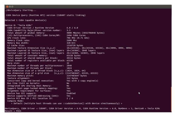
Figure 1: Figure 1. Valid Results from deviceQuery CUDA Sample
