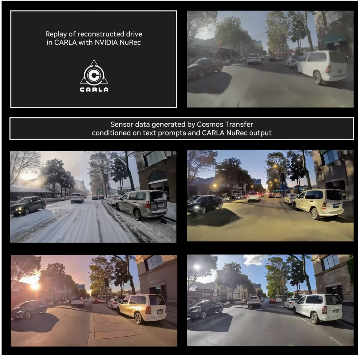
Figure 6: Cosmos Transfer for data coverage of diverse weather & lighting.
