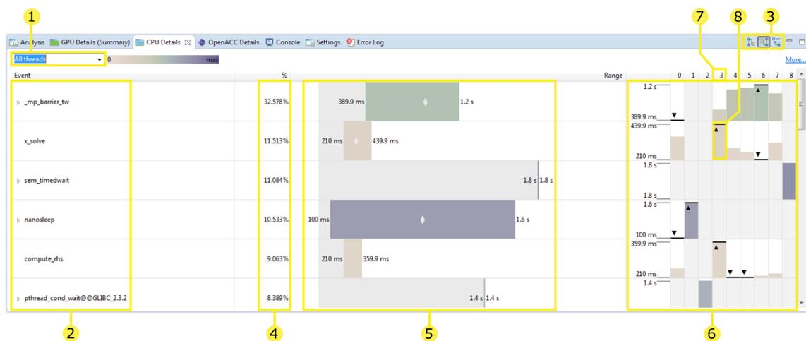
1. All the threads profiled are shown in one view when the 'all threads' option is selected (default). You can use this drop-down menu to instead select an individual thread.
