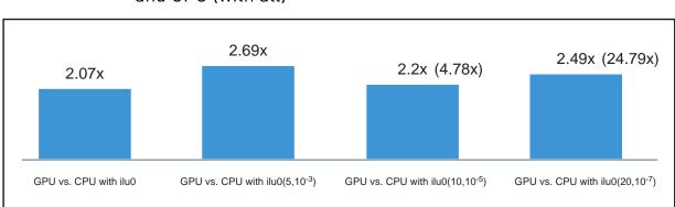
Figure 5. Average Speedup of BiCGStab and CG on GPU (with csrilu0) and CPU (with all)
