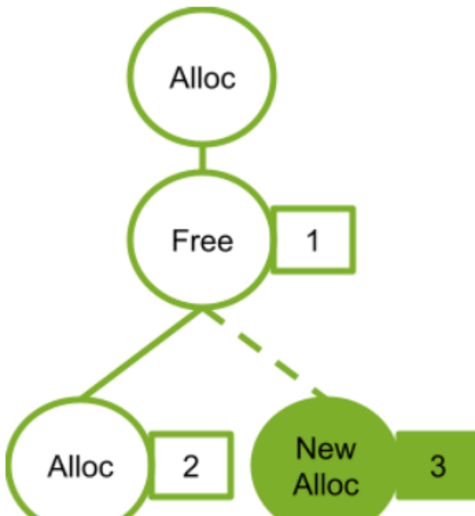
Figure 15. Adding new alloc node 4
