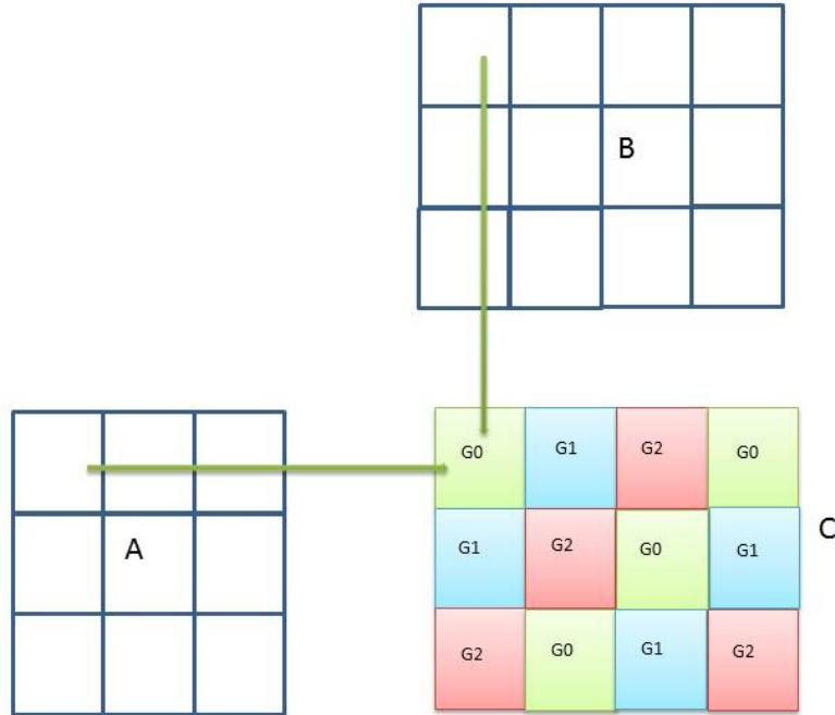
When the tile dimension is not an exact multiple of the dimensions of C, some tiles are partially filled on the right border or/and the bottom border. The current implementation does not pad the incomplete tiles but simply keep track of those incomplete tiles by doing the right reduced cuBLAS operations : this way, no extra computation is done. However it still can lead to some load unbalance when all GPUS do not have the same number of incomplete tiles to work on.
