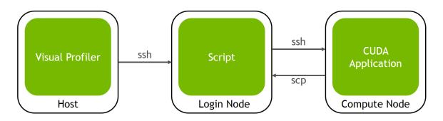
The host machine is the one which is running the Visual Profiler.
