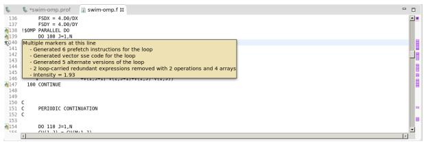
The CPU source code view allows you to inspect the files that comprise the profiled application's CPU source. This view can be opened in the <u>CPU Details View</u> by double-clicking on a function in the tree-the source file that corresponds to this function is then opened. Line numbers can be enabled by right-clicking left side ruler.
