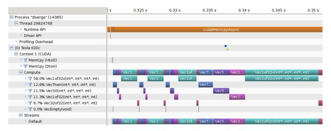
Along the top of the view is a horizontal ruler that shows elapsed time from the start of application profiling. Along the left of the view is a vertical ruler that describes what is being shown for each horizontal row of the timeline, and that contains various controls for the timeline. These controls are described in <u>Timeline Controls</u>
