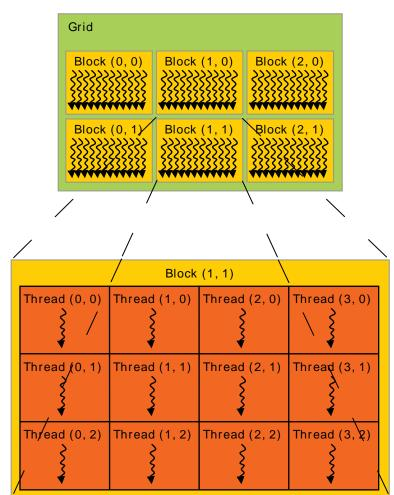
Figure 4. Grid of Thread Blocks
