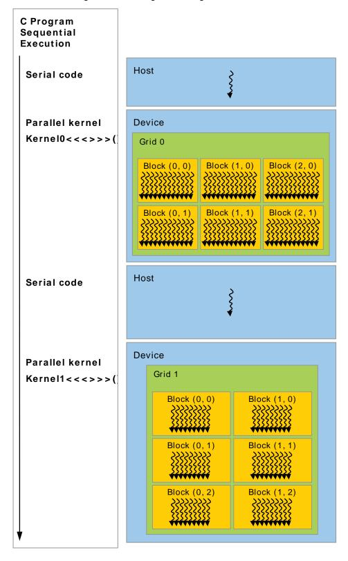
Note: Serial code executes on the host while parallel code executes on the device.
