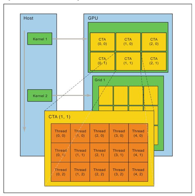
Figure 1. Thread Batching
