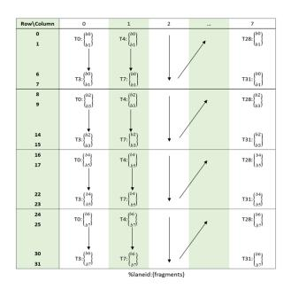
Matrix fragments for accumulators C and D are the same as in case of <u>Matrix Fragments</u> for mma.m16n8k16 with floating point type. Metadata: A .b32 register containing 16 2-bit vectors with each pair of 2-bit vectors storing the indices of two non-zero element from a 4-wide chunk of matrix A as shown below.
