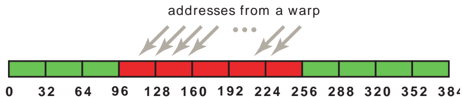
Figure 4. Misaligned sequential addresses that fall within five 32-byte segments
