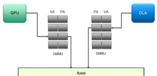
Figure 7. Virtual address to physical address conversion
