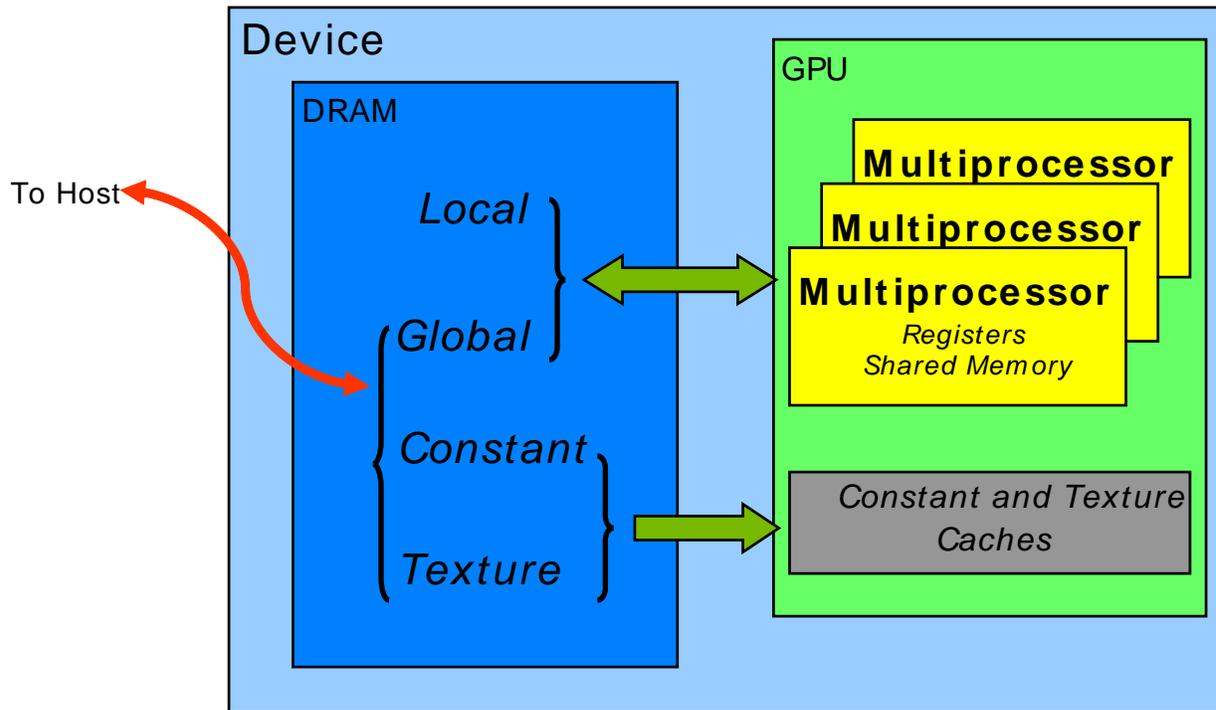
Of these different memory spaces, global memory is the most plentiful; see *Features and Technical Specifications* of the *CUDA C++ Programming Guide* for the amounts of memory available in each memory space at each [compute capability](#) level. Global, local, and texture memory have the greatest access latency, followed by constant memory, shared memory, and the register file.
