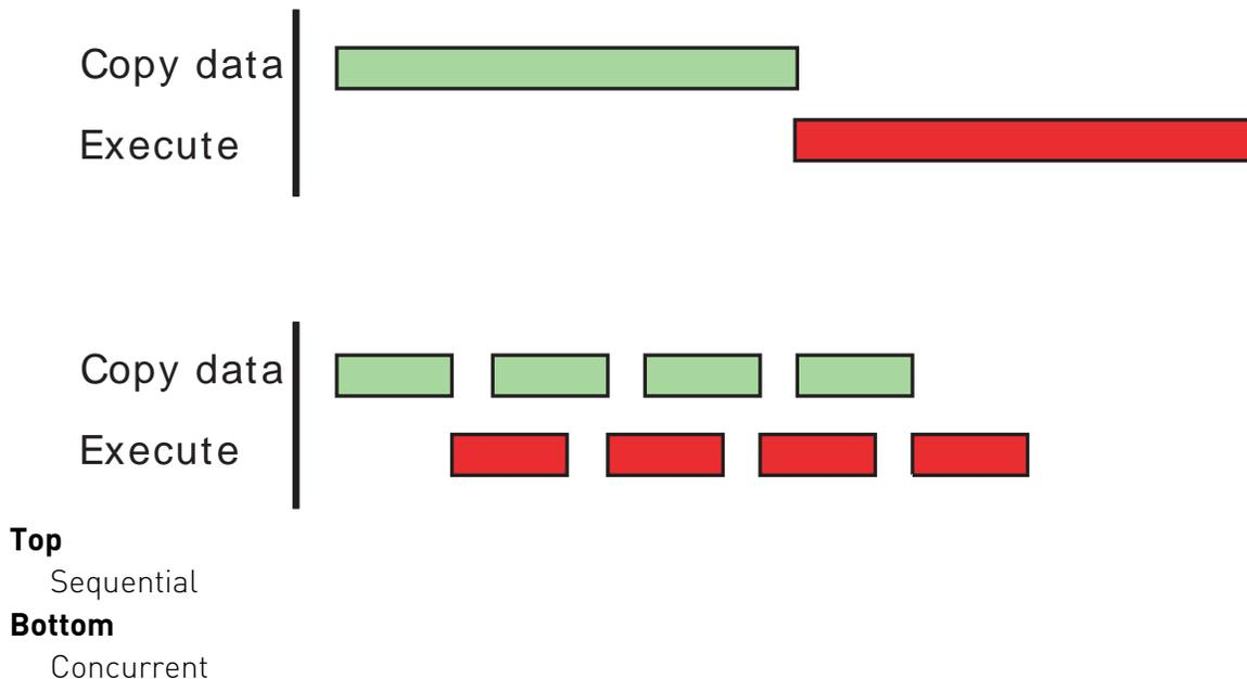
For this example, it is assumed that the data transfer and kernel execution times are comparable. In such cases, and when the execution time ( $t_E$ ) exceeds the transfer time ( $t_T$ ), a rough estimate for the overall time is  $t_E + t_T/nStreams$  for the staged version versus  $t_E + t_T$  for the sequential version. If the transfer time exceeds the execution time, a rough estimate for the overall time is  $t_T + t_E/nStreams$ .
