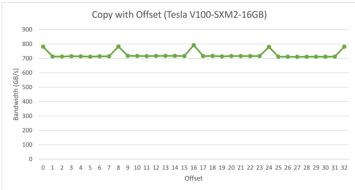
For the NVIDIA Tesla V100, global memory accesses with no offset or with offsets that are multiples of 8 words result in four 32-byte transactions. The achieved bandwidth is approximately 790 GB/s. Otherwise, five 32-byte segments are loaded per warp, and we would expect approximately  $4/5^{\text{th}}$  of the memory throughput achieved with no offsets.
