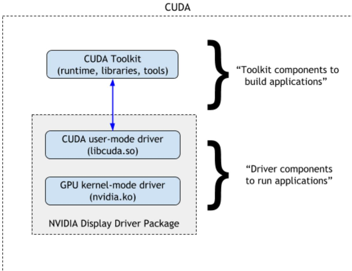
The CUDA compiler (nvcc), provides a way to handle CUDA and non-CUDA code (by splitting and steering compilation), along with the CUDA runtime, is part of the CUDA compiler toolchain. The CUDA Runtime API provides developers with high-level C++ interface for simplified management of devices, kernel executions etc., While the CUDA driver API provides [\[CUDA Driver API\]](#) a low-level programming interface for applications to target NVIDIA hardware.
