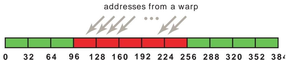
Memory allocated through the CUDA Runtime API, such as via `cudaMalloc()`, is guaranteed to be aligned to at least 256 bytes. Therefore, choosing sensible thread block sizes, such as multiples of the warp size (i.e., 32 on current GPUs), facilitates memory accesses by warps that are properly aligned. (Consider what would happen to the memory addresses accessed by the second, third, and subsequent thread blocks if the thread block size was not a multiple of warp size, for example.)
