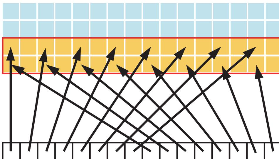
A stride of 2 results in a 50% of load/store efficiency since half the elements in the transaction are not used and represent wasted bandwidth. As the stride increases, the effective bandwidth decreases until the point where 32 32-byte segments are loaded for the 32 threads in a warp, as indicated in [Figure 7](#).
