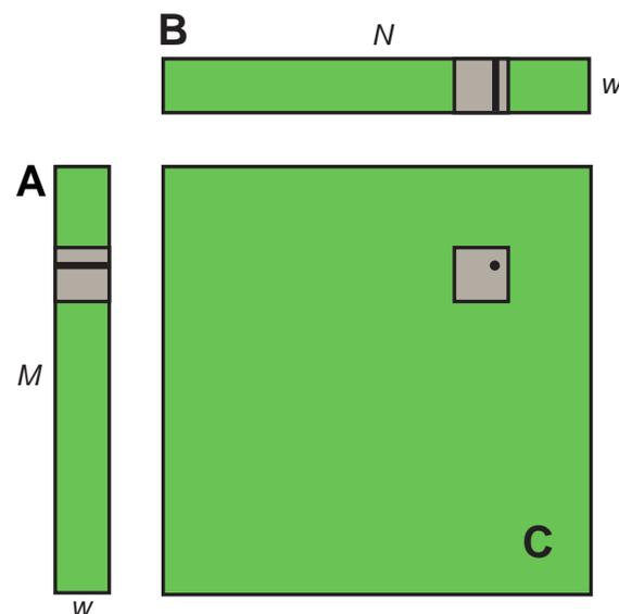
To do this, the `simpleMultiply` kernel ([Unoptimized matrix multiplication](#)) calculates the output elements of a tile of matrix C.
