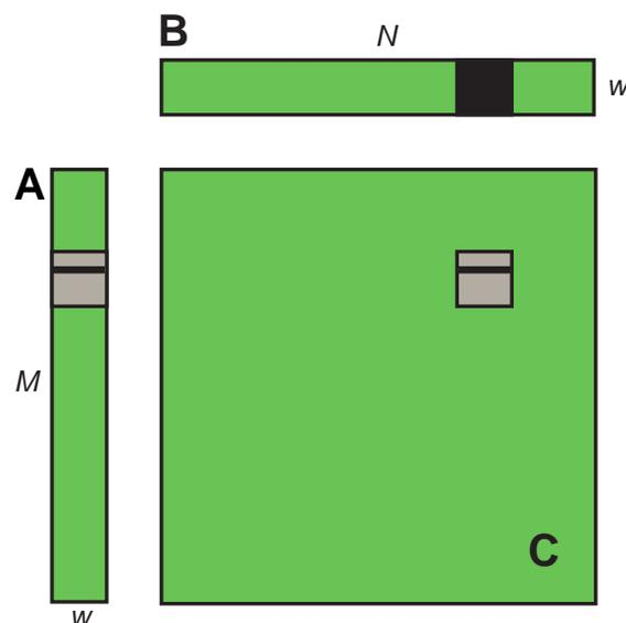
For each iteration  $i$  of the `for` loop, the threads in a warp read a row of the B tile, which is a sequential and coalesced access for all compute capabilities.
