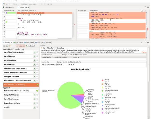
The blog post Pinpoint Performance Problems with Instruction-Level Profiling shows how PC Sampling can be used to optimize a CUDA kernel.
