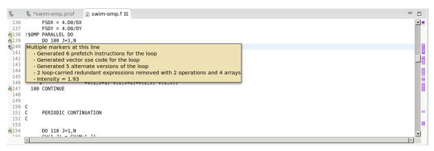
The CPU source code view allows you to inspect the files that comprise the profiled application's CPU source. This view can be opened in the <u>CPU Details View</u> by double-clicking on a function in the tree-the source file that corresponds to this function is then opened. Line numbers can be enabled by right-clicking left side ruler.
