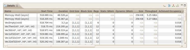
You can sort the data by column by left clicking on the column header, and you can rearrange the columns by left clicking on a column header and dragging it to its new location. If you select a row in the table, the corresponding interval will be selected in the <u>Timeline View</u>. Similarly, if you select a kernel or memcpy interval in the Timeline View the table will be scrolled to show the corresponding data.
