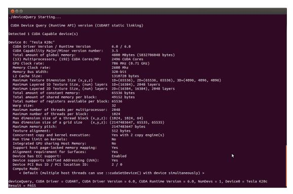
Fig. 1: Figure 1. Valid Results from deviceQuery CUDA Sample
