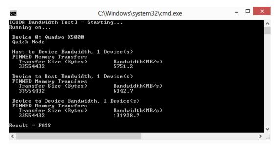
Fig. 2: Figure 2. Valid Results from bandwidthTest CUDA Sample
