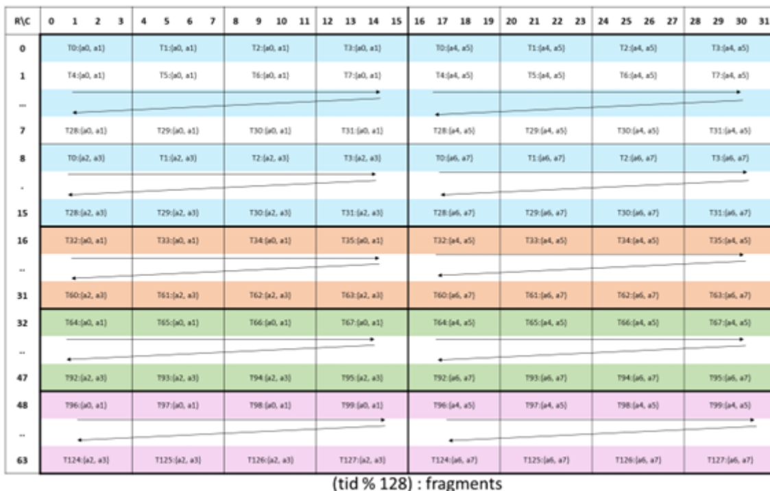
Figure 148: Sparse WGMMA .m64nNk32 fragment layout for matrix A with .f16/.bf16 type.
