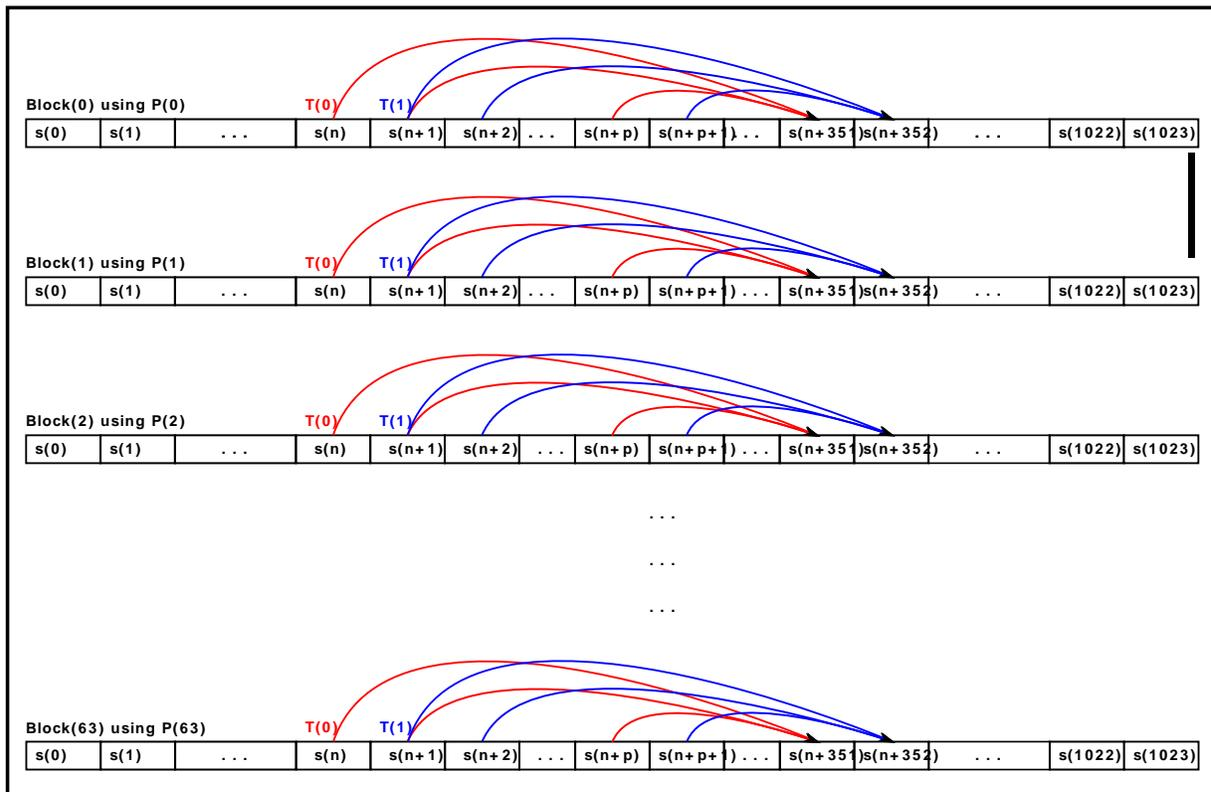
[Figure 1](#) is an illustration of how blocks and threads in MTGP32 operate on the generator states. Each row represents a circular state array of 32-bit integers  $s(n)$ . Threads operating on the array are
