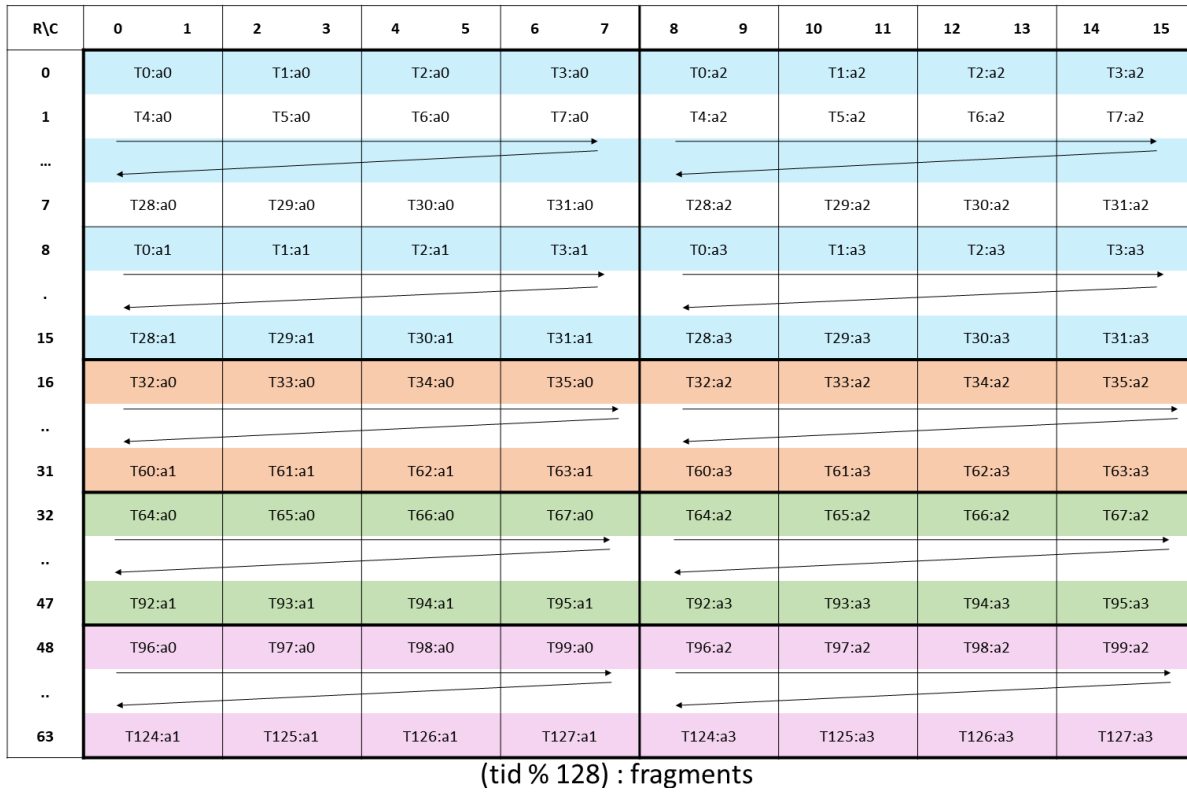
Figure 151: Sparse WGMMA .m64nNk16 fragment layout for matrix A with .tf32 type.
