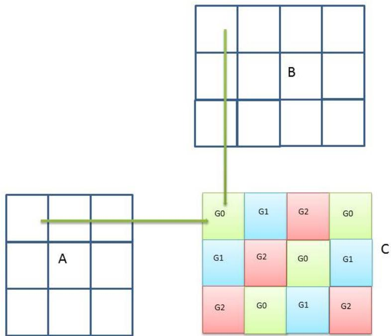
Fig. 1: Example of `cusblasXt<t>gemm()` tiling for 3 Gpus
