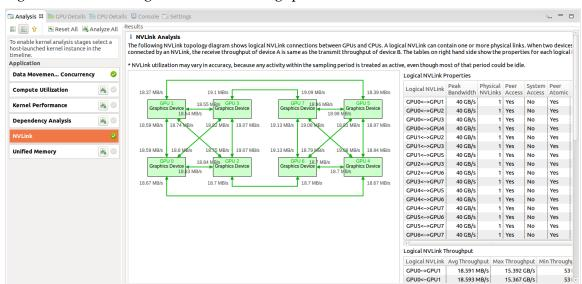
in 'Logical NVLink Properties' table. It also lists the transmit and receive throughputs for logical NVLink in 'Logical NVLink Throughput' table.
