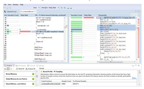
Columns for profiling data collected at the assembly instruction level
