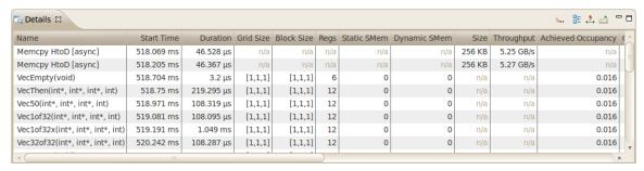
You can sort the data by column by left clicking on the column header, and you can rearrange the columns by left clicking on a column header and dragging it to its new location. If you select a row in the table, the corresponding interval will be selected in the Timeline View. Similarly, if you select a kernel or memcpy interval in the Timeline View the table will be scrolled to show the corresponding data.
