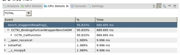
The CPU Details View displays a tree representing the application's execution on the CPU. Each node in the tree can represent a function called by the application. It shows the amount of time spent by the profiled application in the given function. The tree is organized to show the calling hierarchy among functions. The following modes are available:
