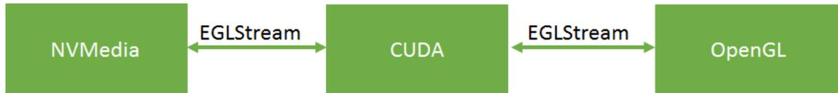
NvMedia and CUDA connect as producer and consumer respectively to one EGLStream. CUDA and OpenGL connect as producer and consumer respectively to another EGLStream.
