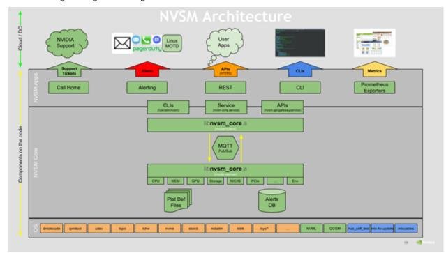
The following is a high level diagram of the NVSM architecture.
