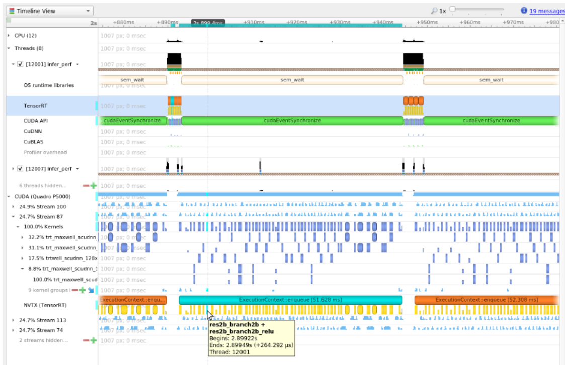
Figure 2 The kernels actually running on the GPU, in other words, it shows the correlation between the layer execution and kernel launch on the CPU side and their execution on the GPU side.
