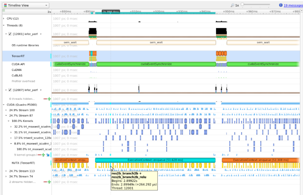
Figure 2. The kernels actually run on the GPU, in other words, it shows the correlation between the layer execution and kernel launch on the CPU side and their execution on the GPU side.
