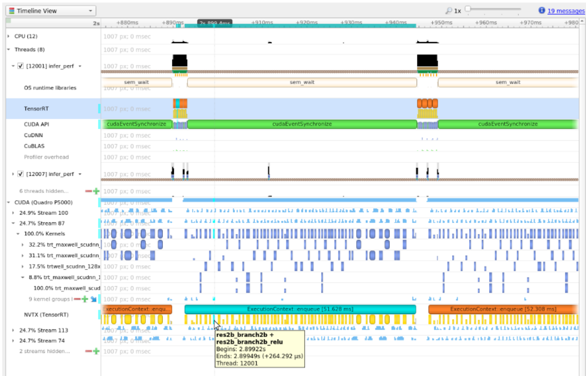
Figure 16. The kernels actually run on the GPU, in other words, it shows the correlation between the layer execution and kernel launch on the CPU side and their execution on the GPU side.
