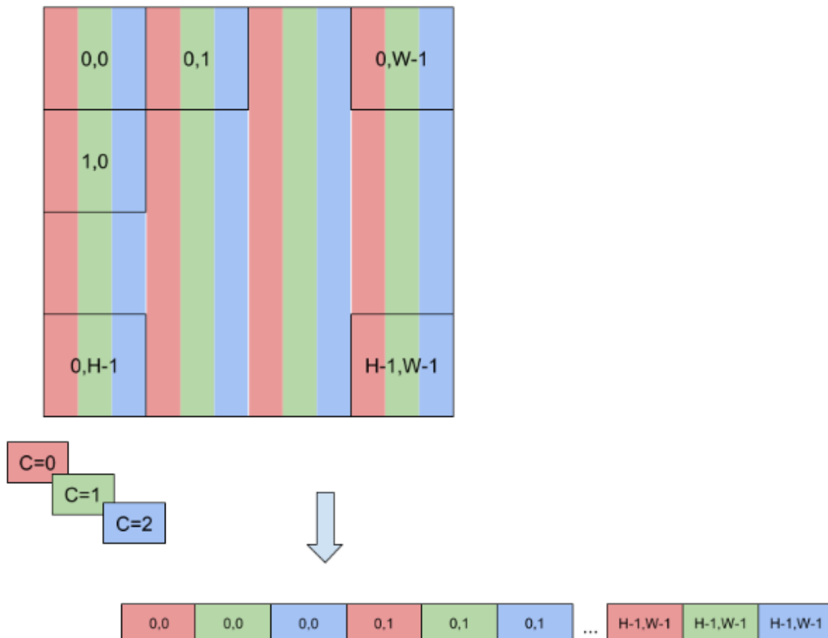
Figure 22. Layout format for HWC : The image is stored as a single H \times W matrix, whose value is actually C -tuple, with a value per channel; all the values of a point (pixel) are stored contiguously.
