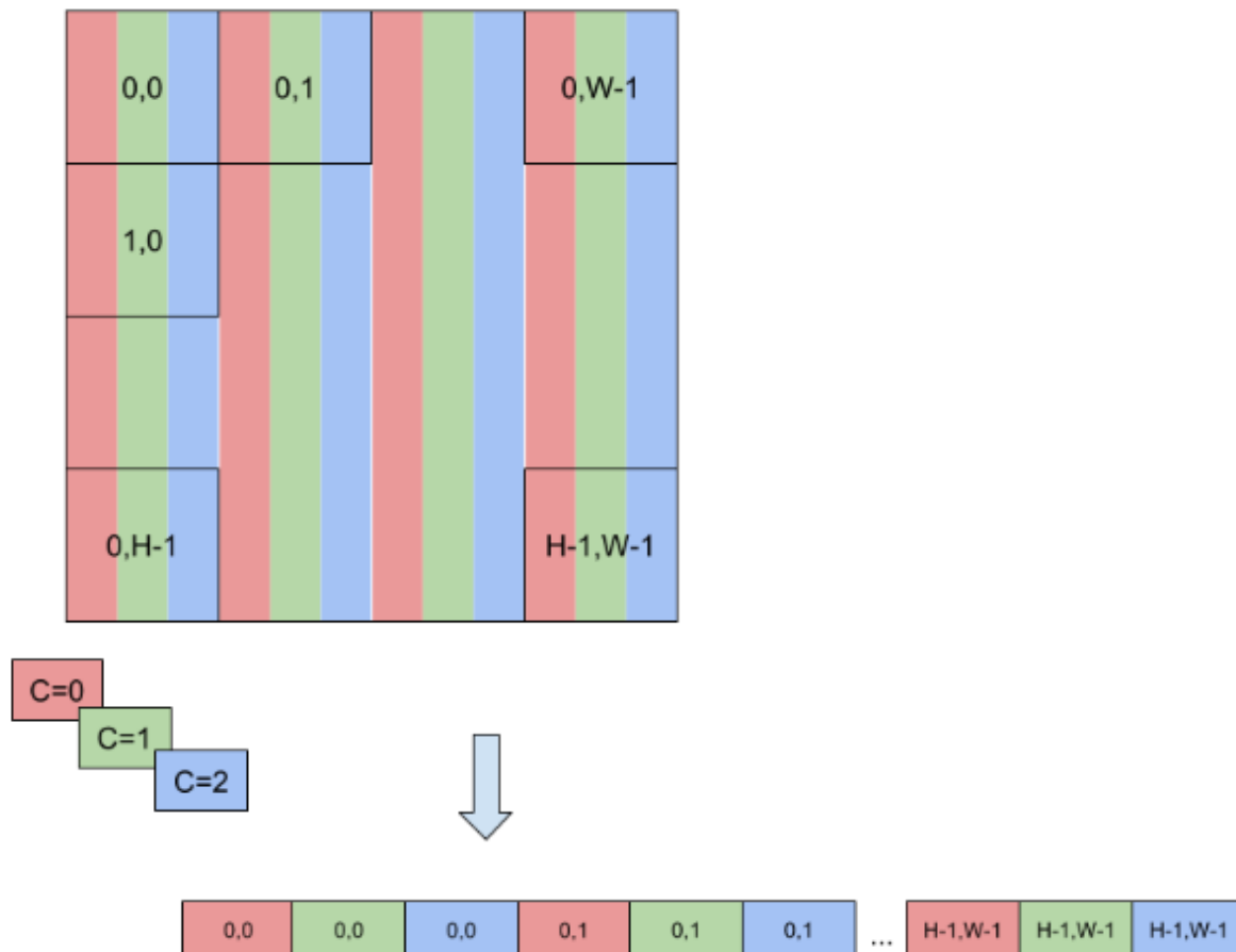
Figure 23. Layout format for HWC : The image is stored as a single H \times W matrix, whose value is actually C -tuple, with a value per channel; all the values of a point (pixel) are stored contiguously.
