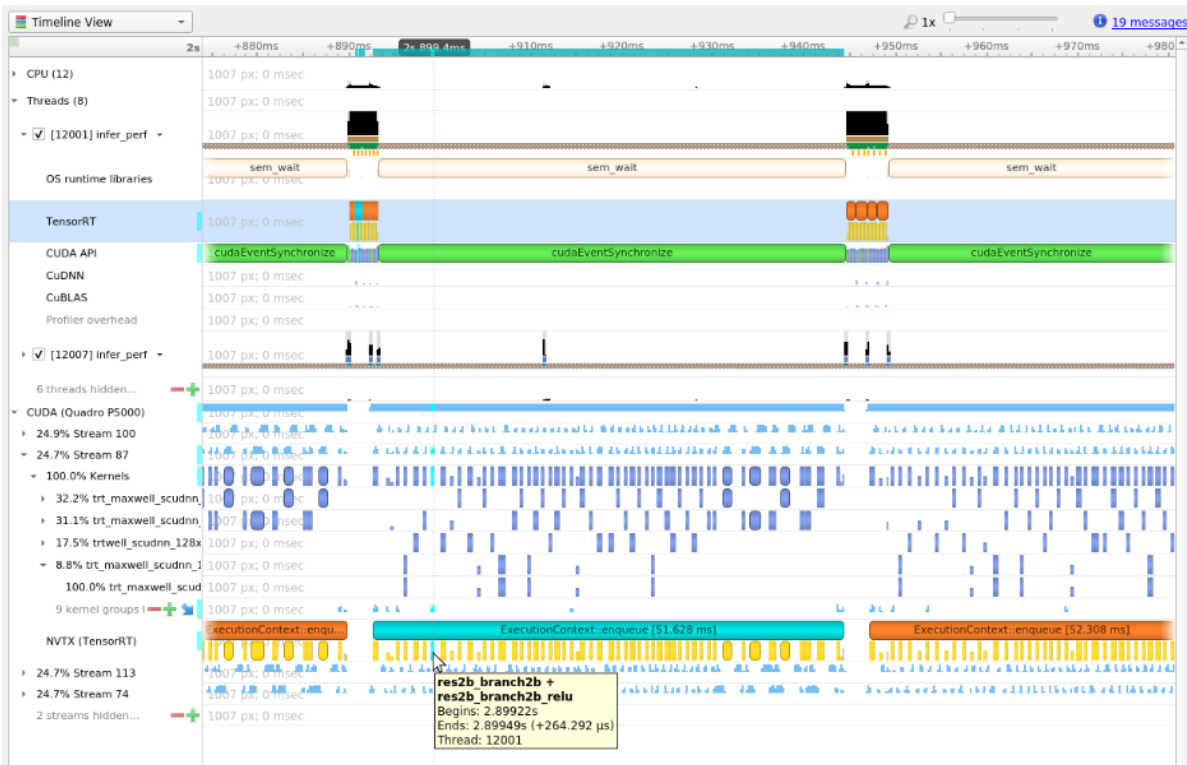
Figure 18. The kernels actually run on the GPU, in other words, it shows the correlation between the layer execution and kernel launch on the CPU side and their execution on the GPU side.
