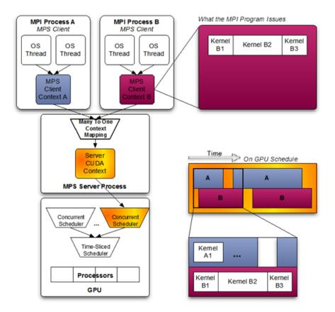
When using pre-Volta MPS, the server manages the hardware resources associated with a single CUDA context. The CUDA contexts belonging to MPS clients funnel their work through the MPS server. This allows the client CUDA contexts to bypass the hardware limitations associated with time sliced scheduling, and permit their CUDA kernels execute simultaneously.
