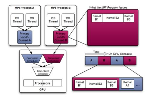
This diagram shows a likely schedule of CUDA kernels when running an MPI application consisting of multiple OS processes without MPS. Note that while the CUDA kernels from within each MPI process may be scheduled concurrently, each MPI process is assigned a serially scheduled time-slice on the whole GPU.
