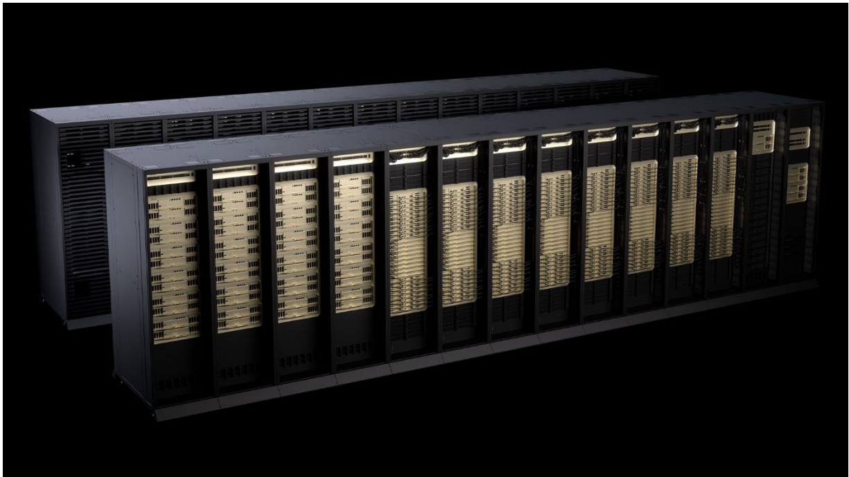
Figure 1. Sample Design for DGX SuperPOD Vera Rubin NVL72
