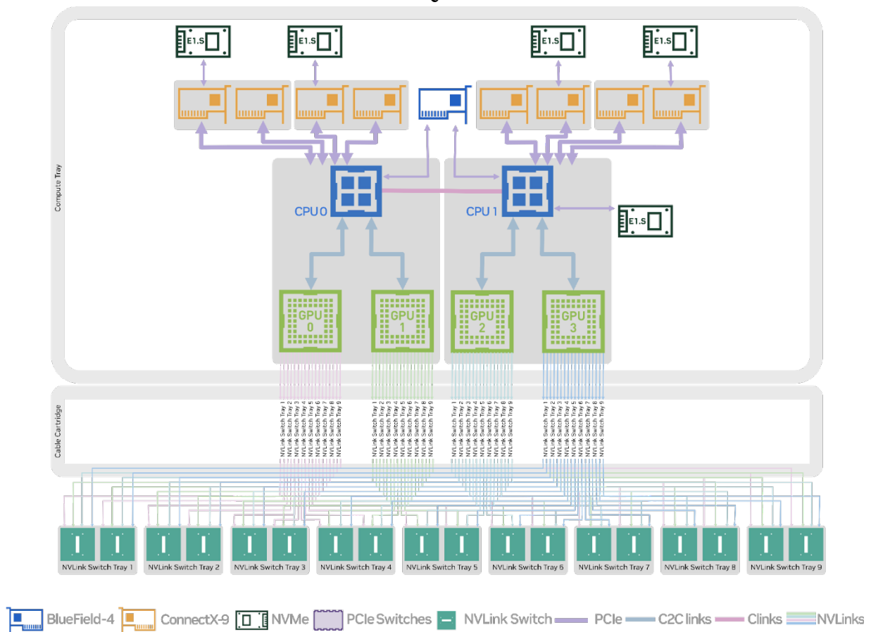
Figure 2. Vera Rubin NVL72 Compute Tray Block Diagram
