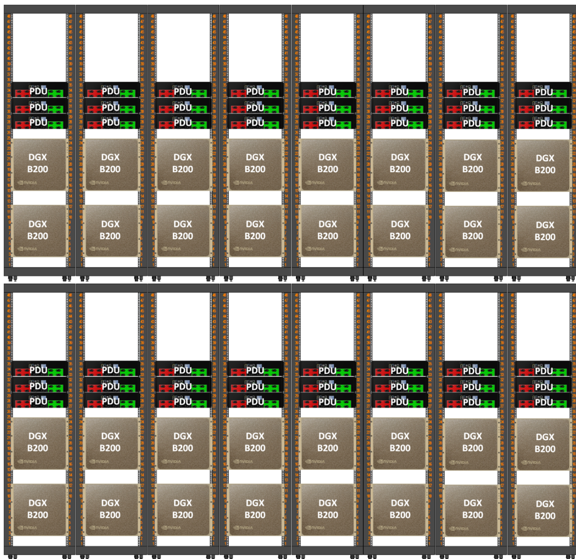
Figure 3.1: Complete single SU rack layout
