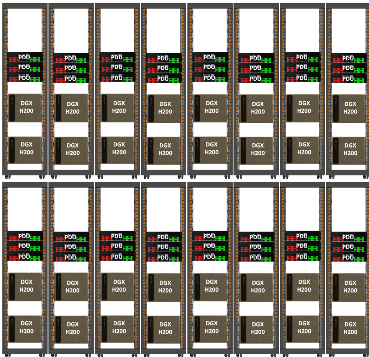
Figure 3.1: Complete single SU rack layout
