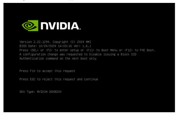
5. Press F10 to accept the BIOS settings and continue to configure SED or disk encryption.
