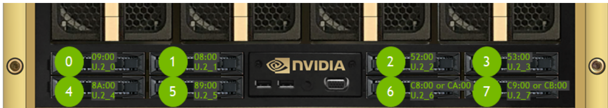
Fig. 1: NVMe Drives: PCIe to Slot Mapping
