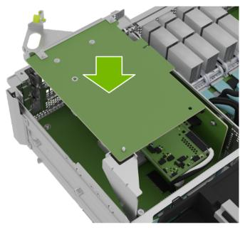
2. Install the M.2 carrier card into the PCI riser by aligning it with the slot and then pressing it against the PCI slot riser:
