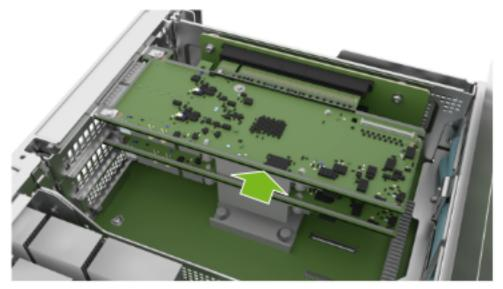
3. Close the latch to lock the PCI cards in place:
