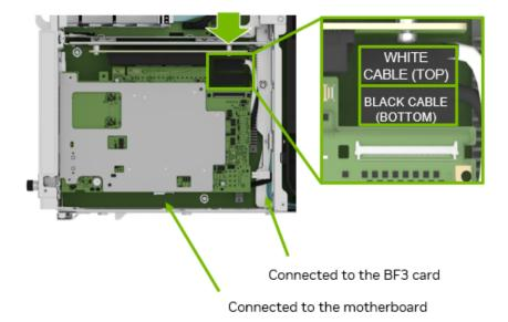
Connect one end of the power cable to the BlueField-3 card and the other end of the power cable to the motherboard.
