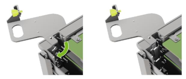
3. Loosen the captive screw on the support bracket of the M.2 riser card:
