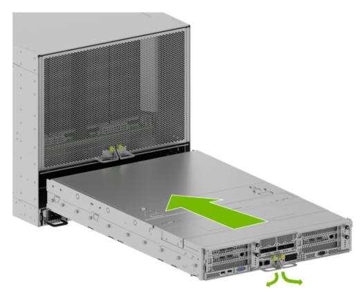
2. Push the motherboard tray into the chassis until the levers on both sides engage with the sides:
