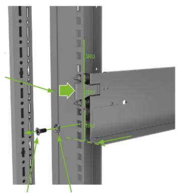
2. Pull on the clip to release the rack mount kit from the post so it can slide back and the prongs can be released from the post.
