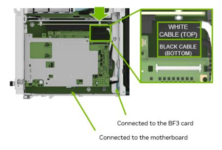
Connect one end of the power cable to the BlueField-3 card and the other end of the power cable to the motherboard.
