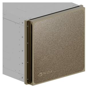
2. Pull the bezel away from the system with a horizontal motion to release it from the magnets that keep it in place.
