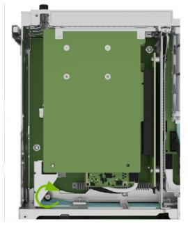
4. Close the latch to secure the M.2 carrier card and secure it in place:
