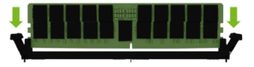
6. To insert the new DIMM, position it in the socket and press down until the levers close and the DIMM clicks into place.
