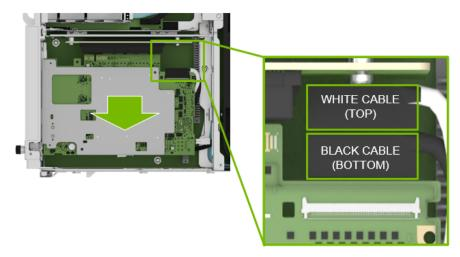
3. Pull the card out of the slot and remove it from the system:
