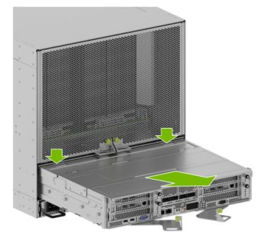
3. Pull the motherboard tray out of the chassis completely:
