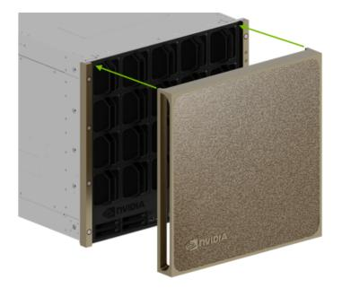
2. Attach the bezel to the system, ensuring that the pins fit in the notches and that the magnetic latch holds the bezel securely in place.
