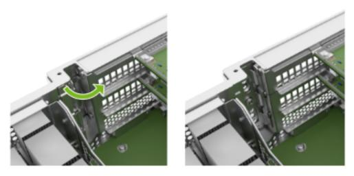
4. Secure the locking mechanism by tightening the black thumbscrew:
