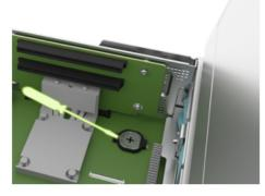
2. Rotate the battery as shown in the following figure:
