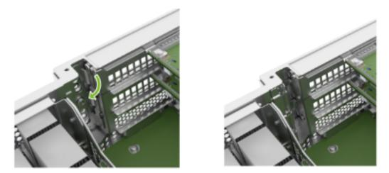
4. Pull the PCI Ethernet card from the slot in the riser:
