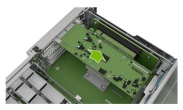
2. Turn the locking mechanism to secure the PCI cards:
