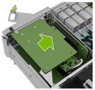
3. Tighten the captive screw on the support bracket of the M.2 PCI riser card:
