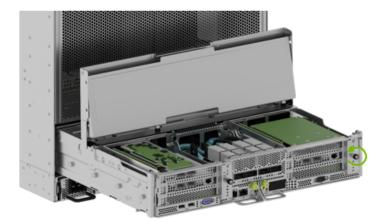
2. Rotate the locking mechanism for the PCI carrier out of the way:
