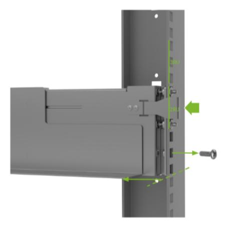
2. Pull on the metal clip and slide the rail away from the post so the progs are free from the rack.
