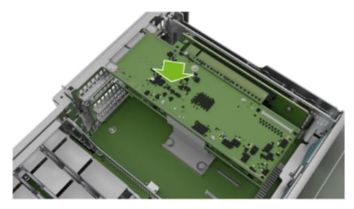
2. Push the card into the PCI slot:
