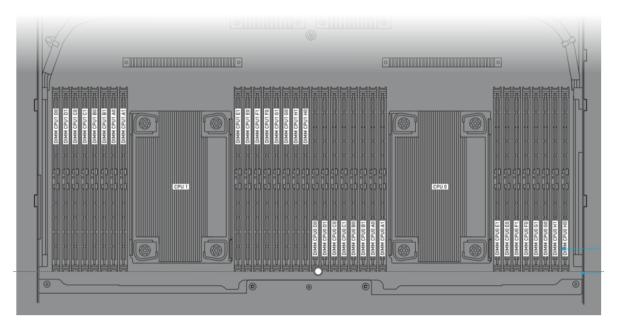
5. To remove the failed DIMM, press down on the ejection levers to eject the DIMM out of the socket.
