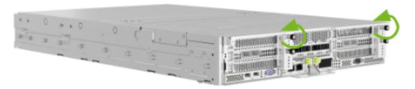
2. Loosen the two screws on the connector side of the motherboard tray, as shown in the following figure:
