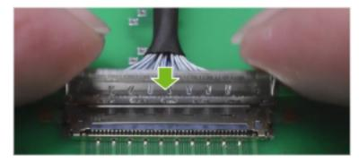
5. Make sure the cable is locked to the connector on the board:
