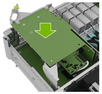
2. Install the M.2 carrier card into the PCI riser by aligning it with the slot and then pressing it against the PCI slot riser:
