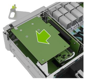
5. Lift the M.2 riser card to remove it from the system:
