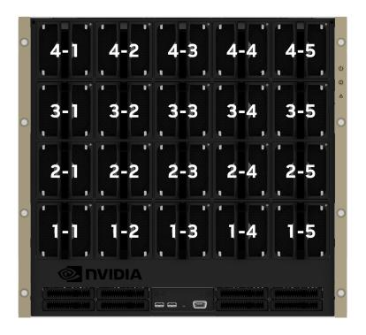
2. Identify the failed fan using the fan module fault LED, as shown in the following figure.
