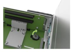
3. Replace the battery with a new CR2032, installing it in the battery holder. Make sure the positive side is on top:
