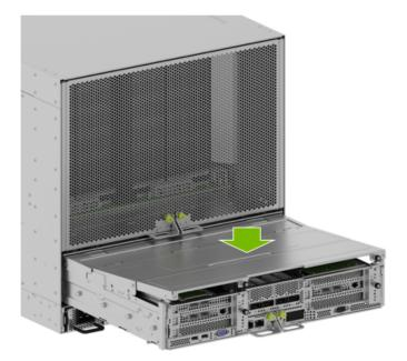
2. Use the thumbscrews indicated in the following figure to secure the lid to the motherboard tray. Open the tray levers:
