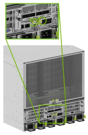
2. Pull the ejection levers to disengage the midplane connectors:
