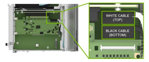
3. Follow the instructions in *Remove an IPEX Cable* to remove the IPEX connectors.
