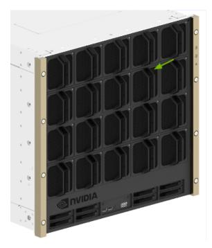
4. Replace the failed fan module with the new one.
