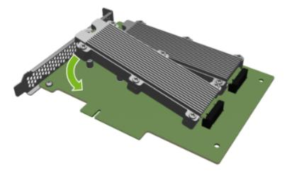
3. Install and tighten the screw to secure the drive to the riser:
