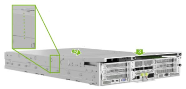
3. Tighten the two lid screws on the port side of the motherboard tray, as shown in the following figure:
