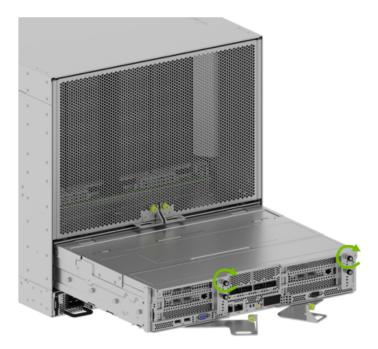
3. Push the motherboard tray into the system chassis until the levers on both sides engage with the sides.
