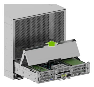
2. Secure the folding section until it stays in place so you can work on the I/O section of the motherboard:
