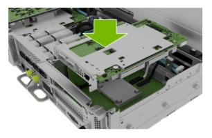
2. Attach the IPEX and power cables as shown in *Insert an IPEX Cable*.
