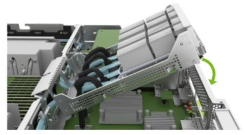
2. Move the OSFP carrier toward the outside of the tray so that the OSFP cages go through the openings on the sheet metal:
