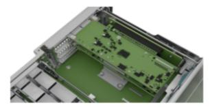
3. Pull the PCI Ethernet card out of the slot:
