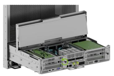
2. Release the PCI cards by turning the locking mechanism 90 degrees as shown in the following figure:
