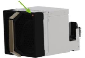
3. Look for the fault LED lit in the upper right corner of the faulty fan module, as shown in the following figure.
