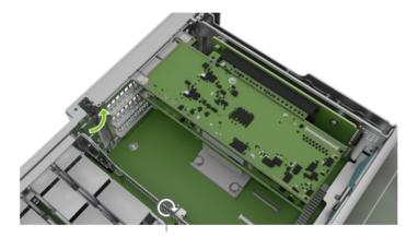
3. Secure the locking mechanism by tightening the black thumbscrew:
