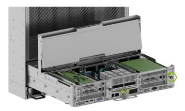
2. Rotate the locking mechanism for the PCI carrier out of the way:
