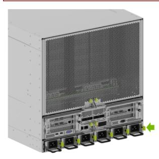
2. Replace the power supply with the new unit making sure the green tab locks into place.
