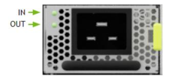
If the PSU is good, both LEDs should be solid green. If either of the LEDs is not green or blinks, contact NVIDIA Enterprise Support to troubleshoot the issue.
