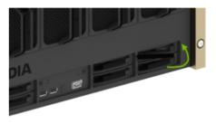
3. Confirm that the drive is flush with the system:
