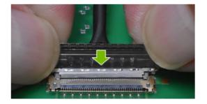
3. Confirm the cable is in the connector:
