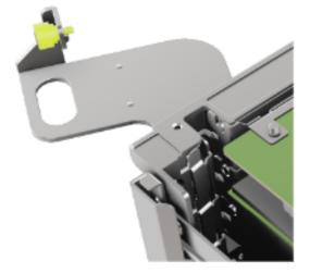
3. Loosen the captive screw on the support bracket of the M.2 riser card:
