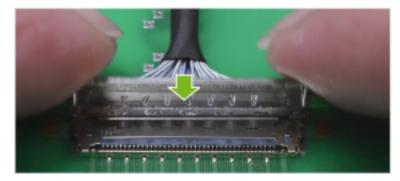
5. Ensure the cable is locked to the connector on the board:
