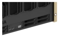
4. Install the bezel after the drive replacement is complete.
