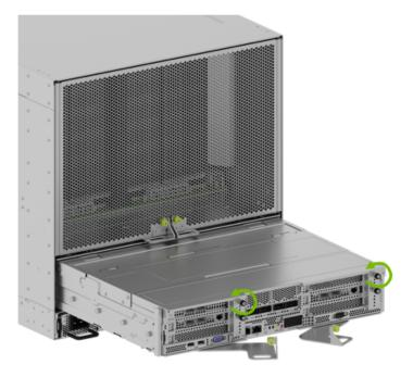
3. Lift the lid I/O section so that it can be folded:
