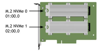
2. Loosen the screw of the identified M.2 drive:
