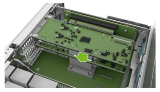
5. Remove the card and prepare the ConnectX-7 card by identifying the IPEX cables that should be removed:
