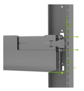
3. Install the round head screw in the rack mount kit to secure it to the post.
