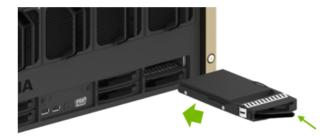
2. Use the handle on the drive to secure it in place:
