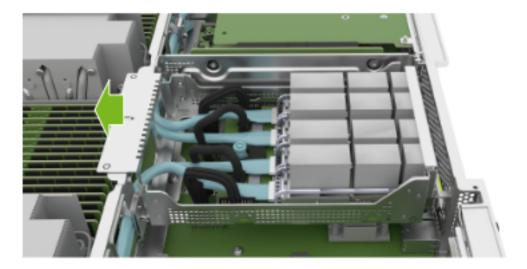
3. Rotate the OSFP carrier module to access the TPM, as shown in the following diagram:
