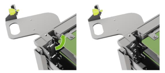
5. Tighten the thumbscrew to ensure the locking mechanism stays in place:
