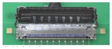
4. Close the latching mechanism:
