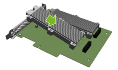
2. Lower the M.2 drive and align it with the screw post:
