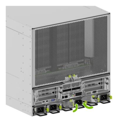
2. After the levers are fully closed, tighten the green thumbscrews to hold the ejection levers in place:
