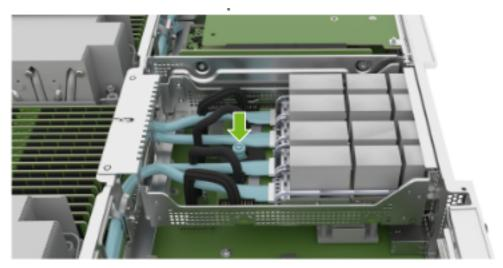
Move the OSFP carrier module toward the DIMMs, as shown in the following figure.
