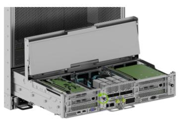
3. Rotate the locking mechanism out of the way to release the PCI cards:
