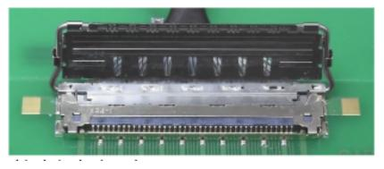
4. Close the latching mechanism:
