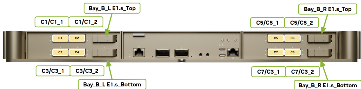
Fig. 3: DGX Vera Rubin NVL72 Compute Tray Networking PCIe Labels Front View
