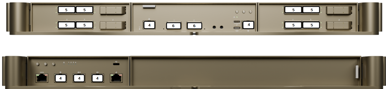
Fig. 1: DGX Vera Rubin NVL72 Compute and Switch Trays - Identification of network port locations
