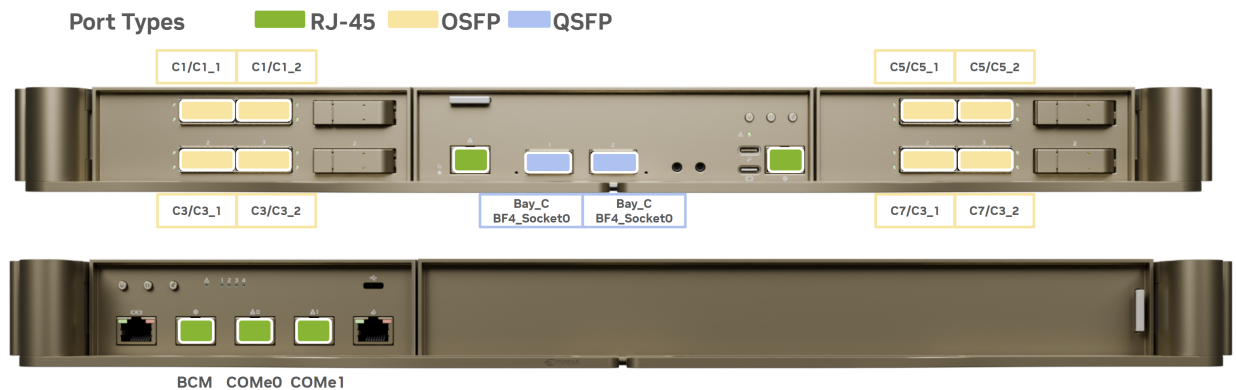
Fig. 2: DGX Vera Rubin NVL72 Compute and Switch Trays - Identification of network port types
