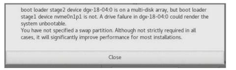
The message appears because the DGX OS from the factory has created a RAID 1 array for the root partition, and has replicated the EFI system partitions.
