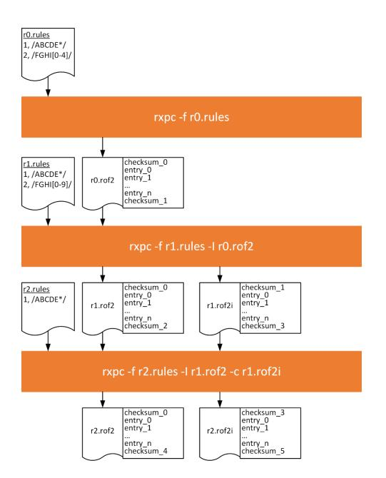
In this figure, r0.rules is the original ruleset or revision zero. This is compiled in the normal way resulting in r0.rof. The "[0-4]" class in rule id two is then changed to "[0-9]" resulting in r1.rules (revision one). In order to incrementally update the RXPs rules memories for each new revision the incremental compile feature can be used. It can be seen that r1.rof2i is the result of incrementally compiling r1.rules using r0.rof2 as a baseline.
