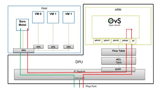
The red arrow demonstrates a packet flow through the representors, while the green arrow demonstrates the packet flow when steering rules are offloaded to the embedded switch. More details on that are available in the switch offload section.
