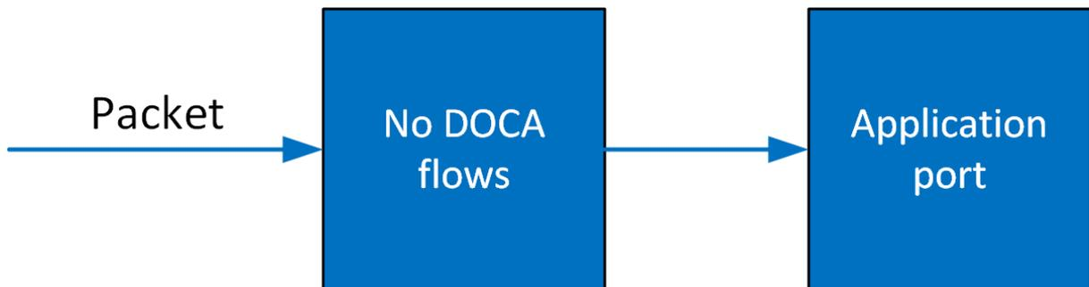
Once entries are added to the PIPE, if a packet has no match then it continues to the port in the software. If it does match, then the rules defined in the PIPE are executed.
