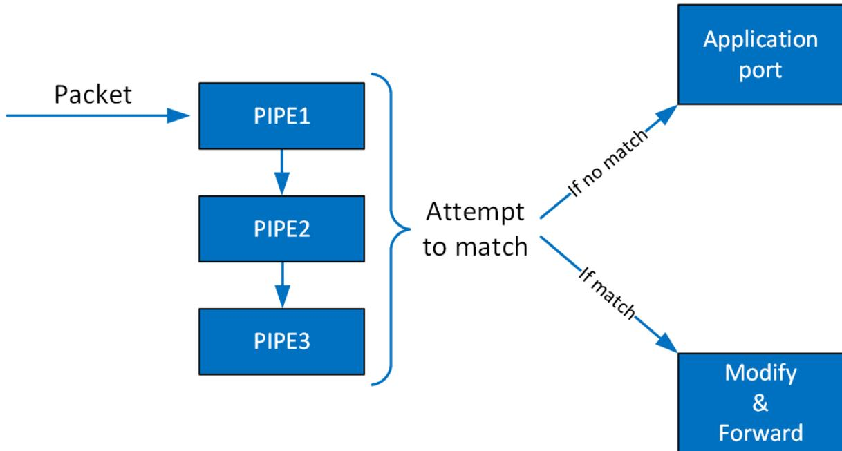
If the packet is forwarded in RSS, the packet is forwarded to software according to the RSS definition. If the packet is forwarded to a port, packet is redirected back to the wire. If the packet is forwarded to the next PIPE, then the software attempts to match it with the next PIPE.
