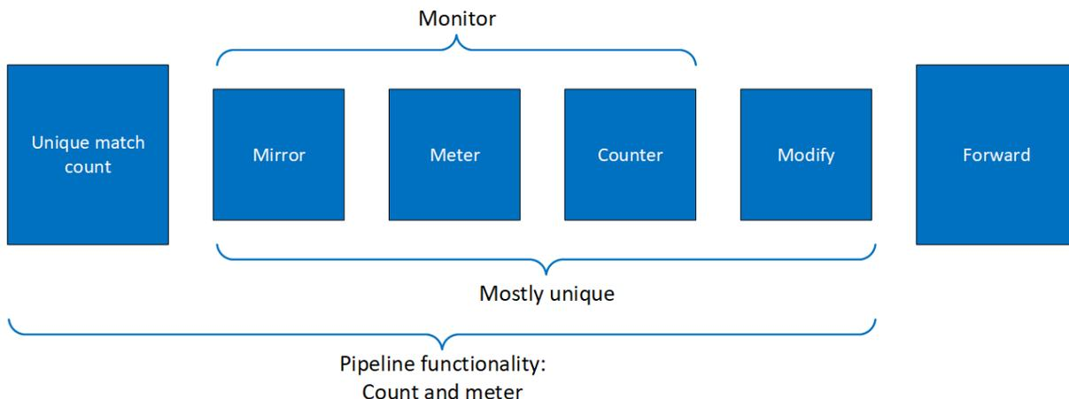
The creation phase allows the HW to efficiently build the execution PIPE. After the PIPE is created, specific entries can be added. Only a subset of the PIPE can be used (e.g. skipping the monitor completely, or just using the counter, etc).
