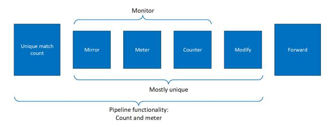
The creation phase allows the HW to efficiently build the execution pipe. After the pipe is created, specific entries can be added. Only a subset of the pipe can be used (e.g. skipping the monitor completely, just using the counter, etc).
