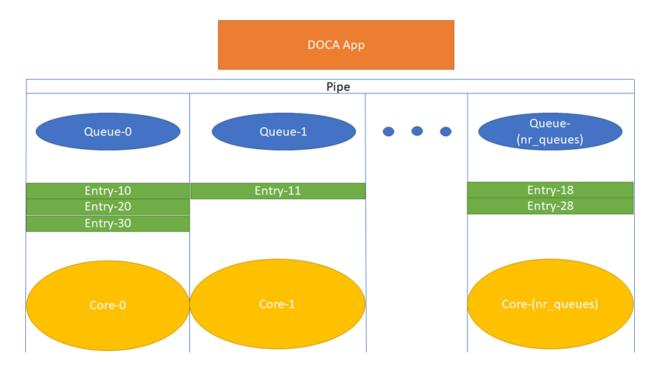
Each core is expected to use its own dedicated pipe\_queue number when calling doca\_flow\_pipe\_entry. Using the same pipe\_queue from different cores causes a race condition and has unexpected results.
