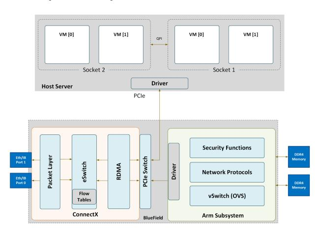
For each one of the BlueField DPU network ports, there are 2 physical PCIe networking functions exposed.
