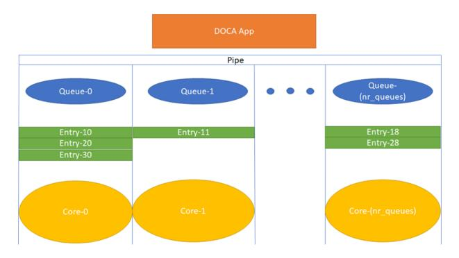
Each core is expected to use its own dedicated pipe queue number when calling doca flow pipe entry. Using the same pipe queue from different cores causes a race condition and has unexpected results.
