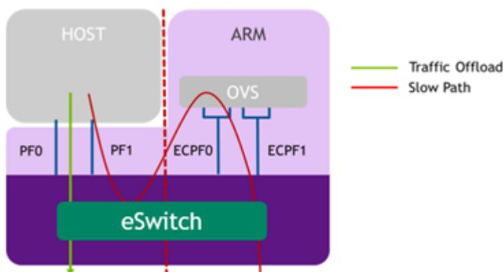
When the server and DPU are initiated, the networking to the host is blocked until the virtual switch on the DPU is loaded. Once it is loaded, traffic to the host is allowed by default.
