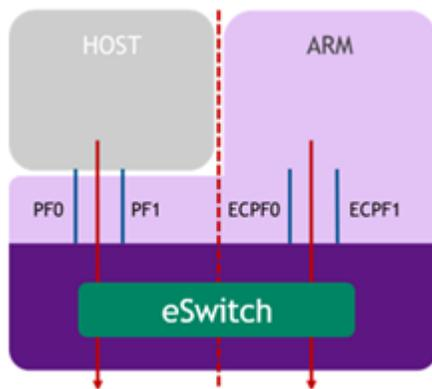
This mode enables the same operational model of a SmartNIC (that does not have a separated control plane). In this case, the Arm control plane can be used for different functions but does not have any control on the host steering functions.
