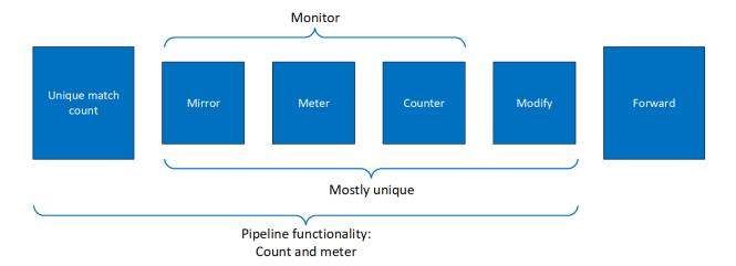
The creation phase allows the HW to efficiently build the execution pipe. After the pipe is created, specific entries can be added. Only a subset of the pipe can be used (e.g. skipping the monitor completely, just using the counter, etc).
