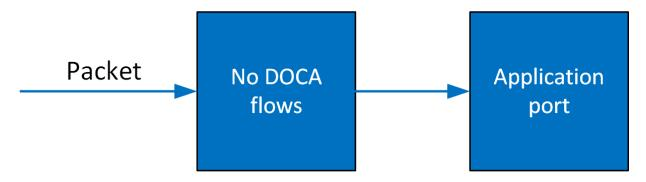
Once entries are added to the pipe, if a packet has no match then it continues to the port in the software. If it is matched, then the rules defined in the pipe are executed.
