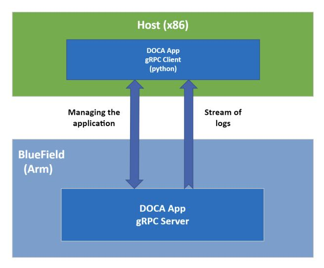
For this purpose, DOCA now includes built-in gRPC support, thereby exposing to the host the application's logical interface in the form of a gRPC-equivalent API.
