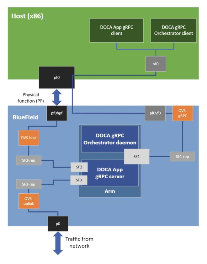
As can be seen above, the application is a bump-on-the-wire, and the gRPC-related traffic flows through a separate OVS bridge connected to the host using a virtual function (VF). More
