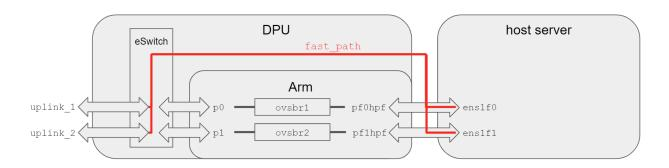
As seen in the following figure, the default configuration for HBN is different: There is only one bridge, and the bridge is only connected to the port representatives, pf0hpf and pf1hpf.
