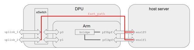
After applying the mlxconfig command (on host server or the DPU) and rebooting the host server, the following diagram represents the default HBN configuration:
