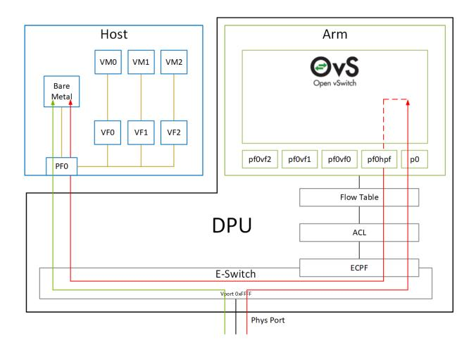
The red arrow demonstrates a packet flow through the representors, while the green arrow demonstrates the packet flow when steering rules are offloaded to the embedded switch. More details on that are available in the switch offload section.
